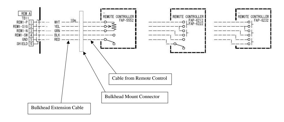
Note – If the remote controllers are connected directly to the processor unit and this extension cable is not used, refer to the applicable color codes in the interconnect diagram in Navpilot installation manual.
